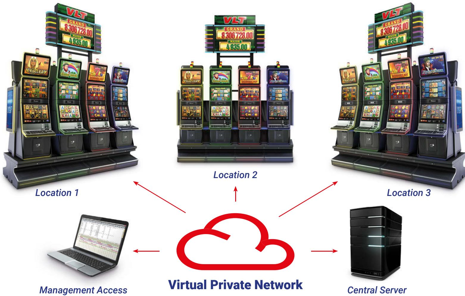
The *Global Solution VLT* is a server-based system that comprises two main components – *Central Server* and *Locations*. The number of locations that can be connected to the *Central Server* is unlimited.
